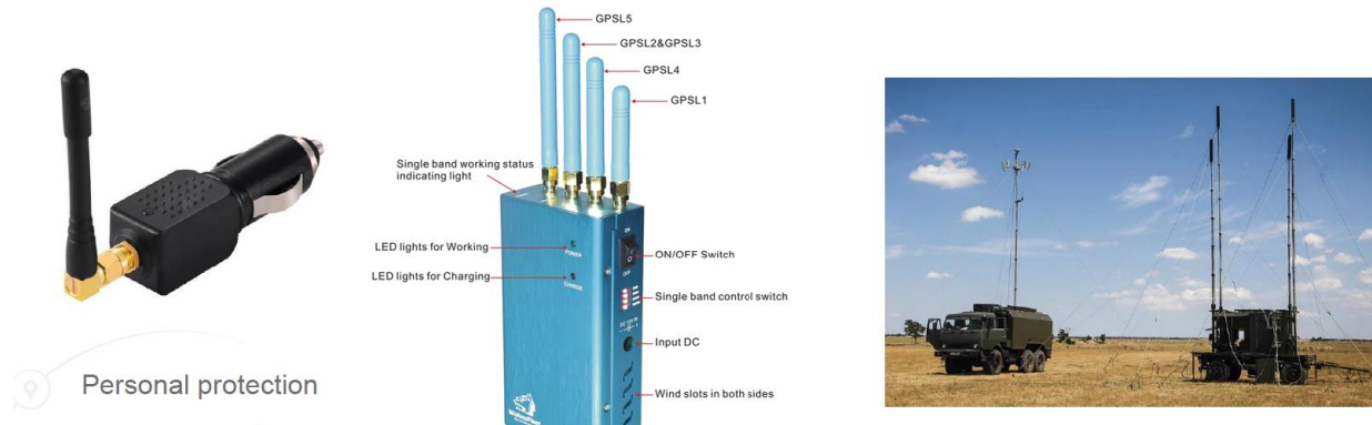
Figure 1. Various jamming systems. (left) A personal protection device, (middle) a car GPS jammer, (right) a military jamming system [7].
