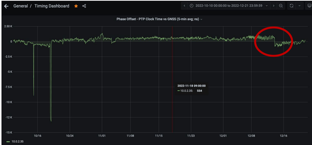
Figure 2: Two-month plot of phase offset data between SRNL BC and GPS.
