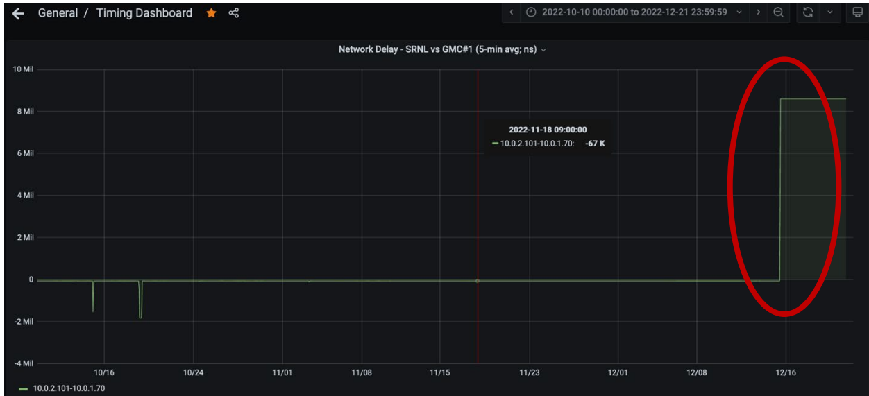
Figure 3: Two-month plot of one-way network latency between SRNL BC and ORNL GMC.
