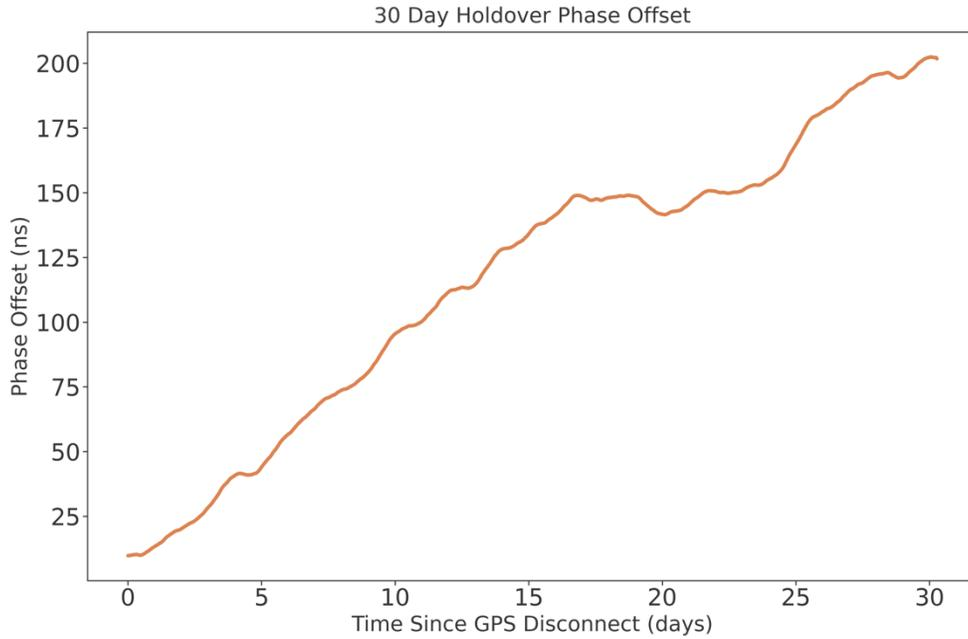
Figure 3. Phase Offset Results from 30 Day Holdover Test
