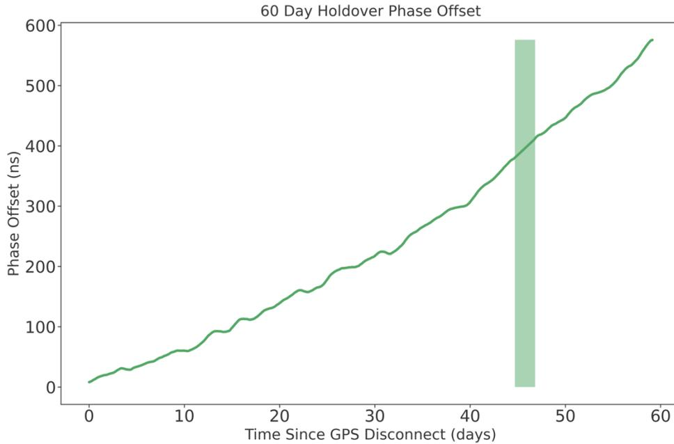
Figure 4. Phase Offset Results from 60 Day Holdover Test
