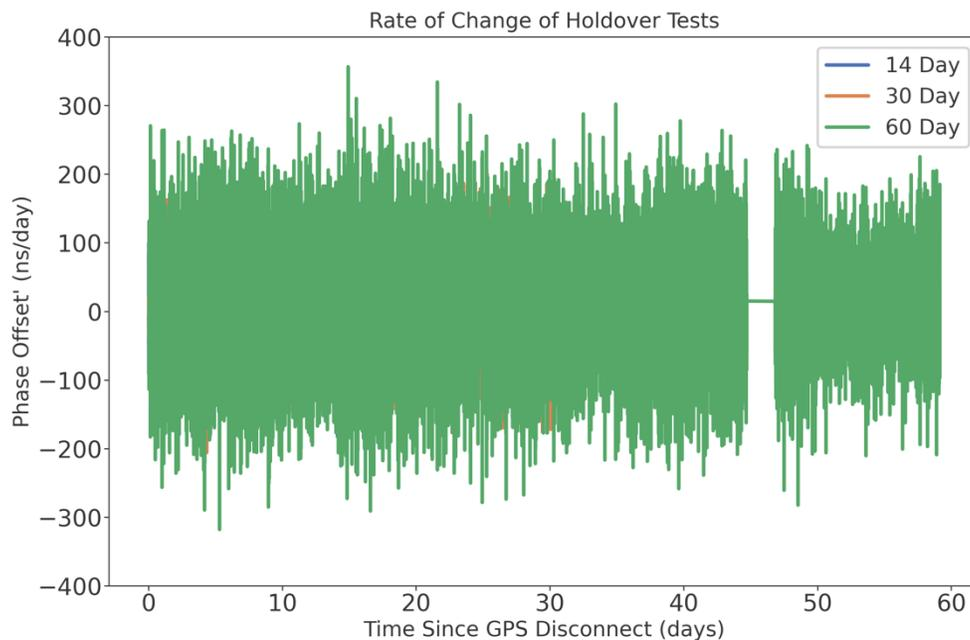
Figure 6. Phase Offset Rate of Change for All Holdover Tests
