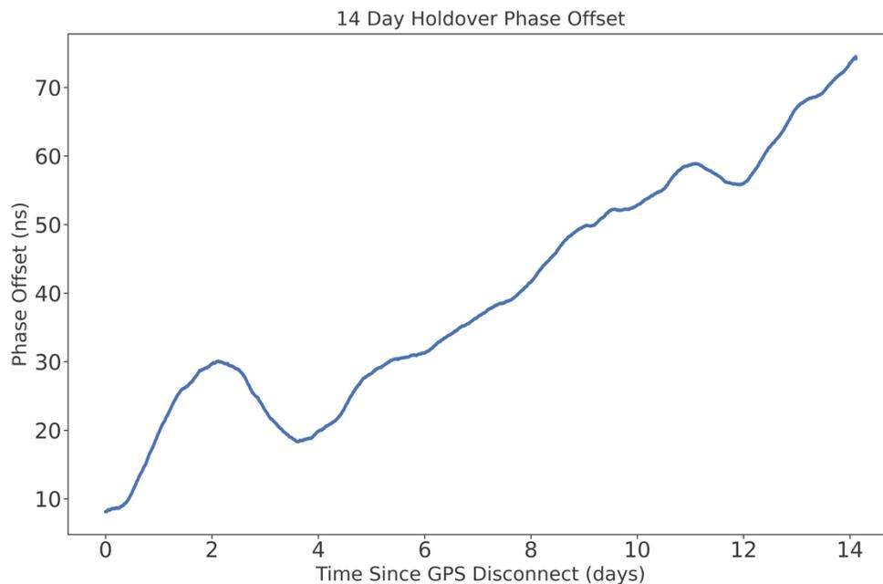
Figure 2. Phase Offset Results from 14 Day Holdover Test
