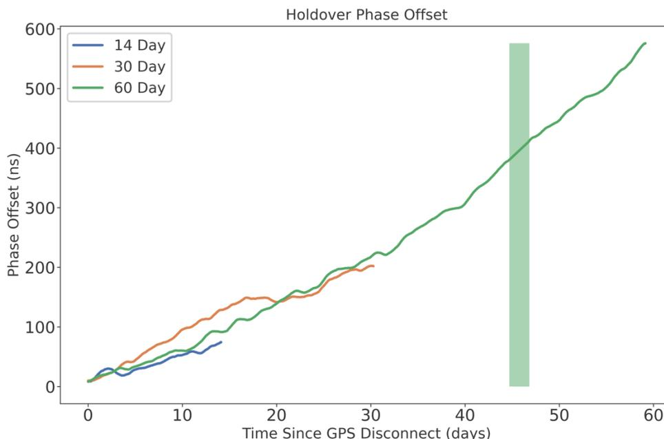
Figure 5. Phase Offset of all Three Holdover Tests
