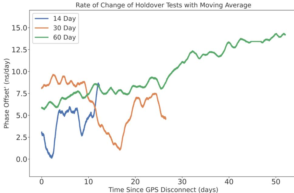
Figure 7. Phase Offset Rate of Change for All Holdover Tests with Moving Average
