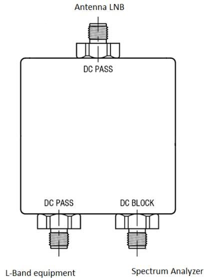
**Figure 3. Splitter to connect the spectrum analyzer.**
