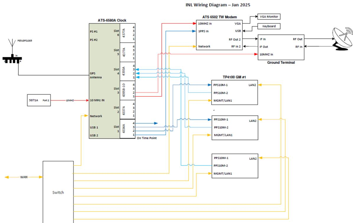
Figure 6. TWSTFT wiring diagram
