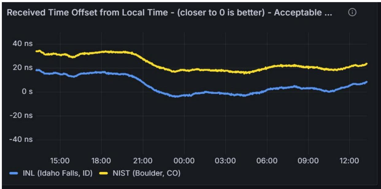
Figure 8. TWSTFT INL time offset compared to NIST.
